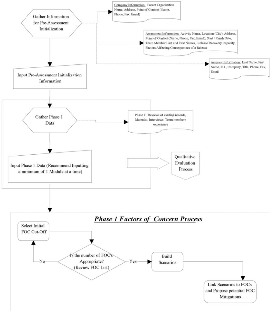
**Figure C-1 - SMAS Data Management Tool Process Diagram (Pre-Assessment & Phase 1)**
