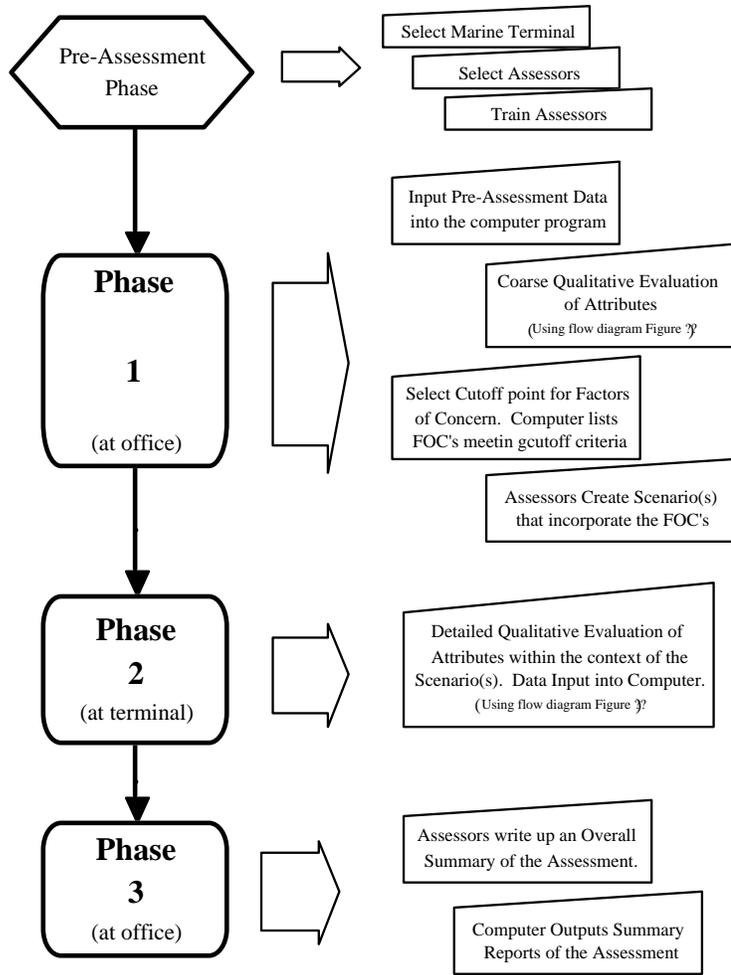
**Figure 3: SMAS Process Flow Diagram**
