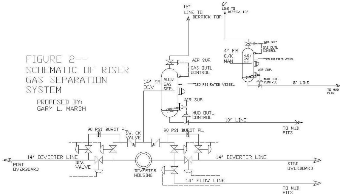
Figure 6.2 – Schematic of riser gas separation system, Proposed by Gary L. Marsh
