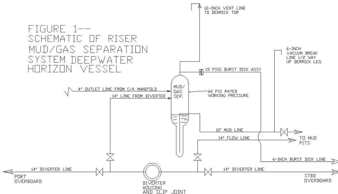
**Figure 5.1 – Schematic of a riser mud/gas separation system Deepwater Horizon vessel<sup>1</sup>**
