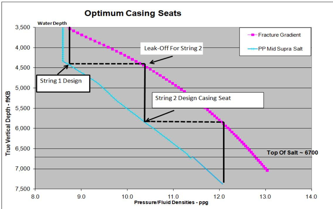
Figure 7.2 – Optimum casing seats maximizing the uncertainty of the drilling margin<sup>iv</sup>
