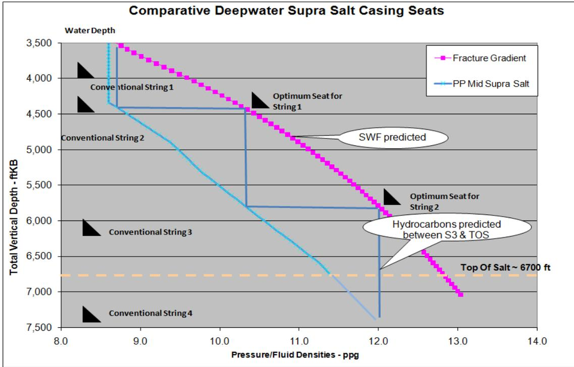
Figure 7.3 – Conventional vs. optimum casing seats: stacking vs. optimum.<sup>v</sup>
