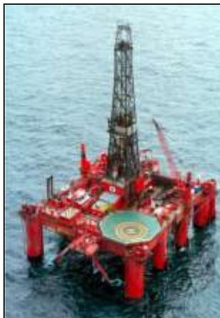
Figure 4.3 – Aker H-3 design semisubmersible *Treasure Seeker*.<sup>17</sup>
