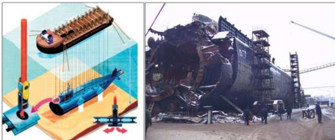
**Figure 3.6 – Illustration of the lifting connection used to salvage the Kursk.<sup>13</sup>**
