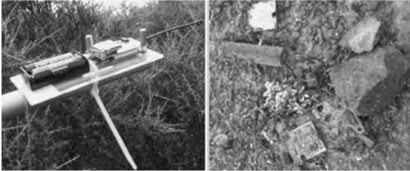
Fig. 14. A Weather Sensor Mote Before and After a Burn.
